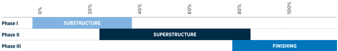
Figure 2: A case study of the construction timeline for a mid-rise steel frame high school. (Riley, 2011)
