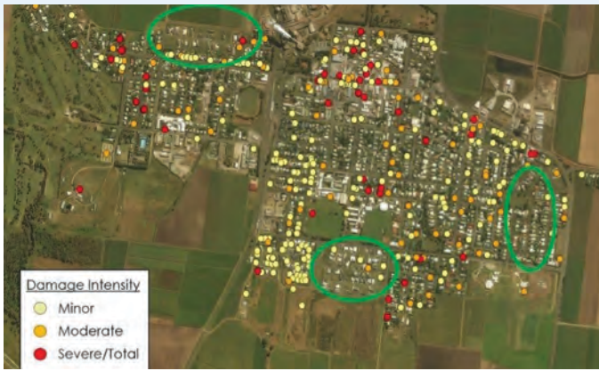
Figure 3: (Left) RDA data collected by QFES and NSW SES in Proserpine following TC Debbie. (Right) Total loss ratio (building + contents) in Proserpine for all insurers following TC Debbie. Note: Areas within green ellipses show claims for modern housing where RDA data did not identify damage had occurred to the building exterior.
